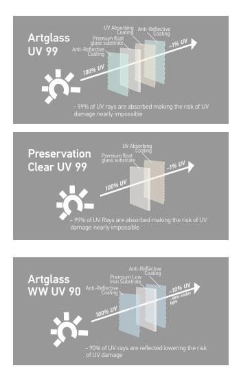
Artglass UV 99<sup>™</sup> is coated on both sides – a very special anti-reflective coating is applied on both surfaces offering the supreme clarity only possible from Groglass<sup>®</sup>. One of the sides is additionally coated with an absorptive UV filter, which is applied by vacuum and specialty roller to leave no sign of distortion or interference. The result is a clear super transparent conservation grade class.
